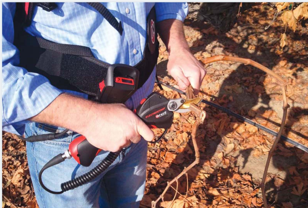
The battery pack allows for two full days of pruning before recharging.
