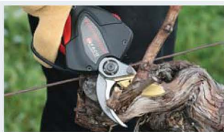
The Electrocoup pruners from Infaco have quick-change cutting heads for cuts from 35 mm to 55 mm.
